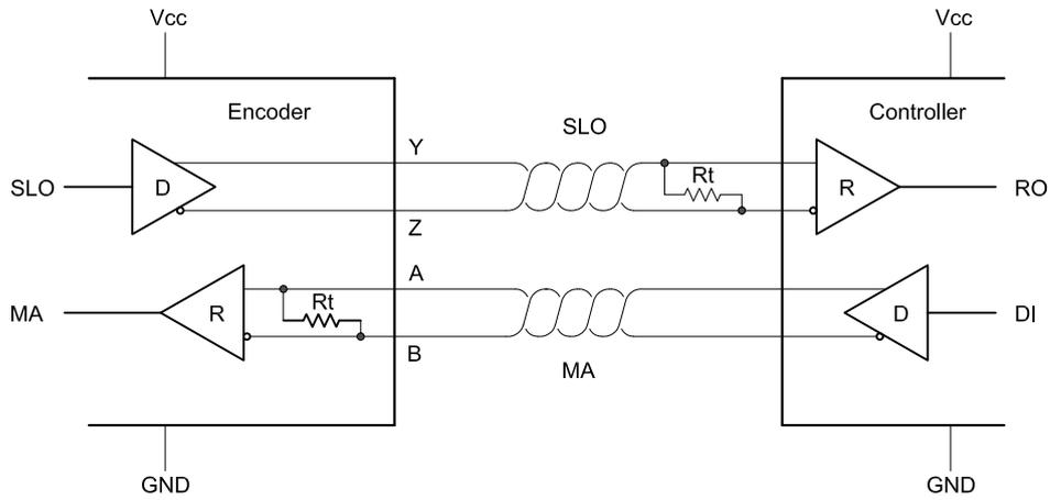
Figure 1: Point-to-point configuration
